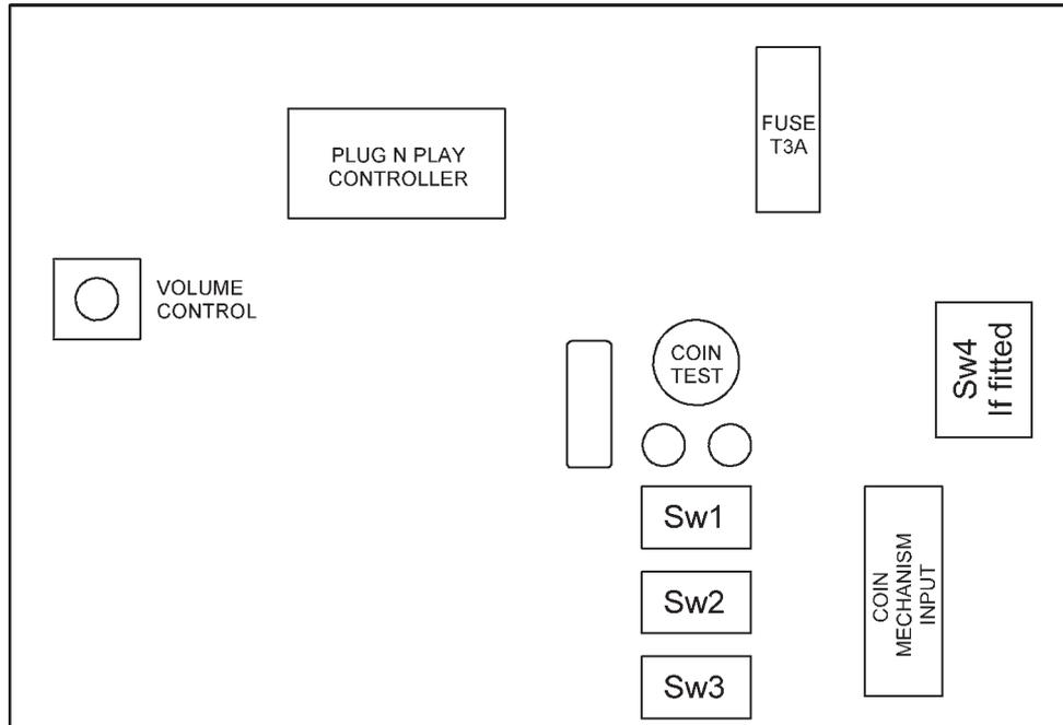
Fig 1 Programmable Control Unit
