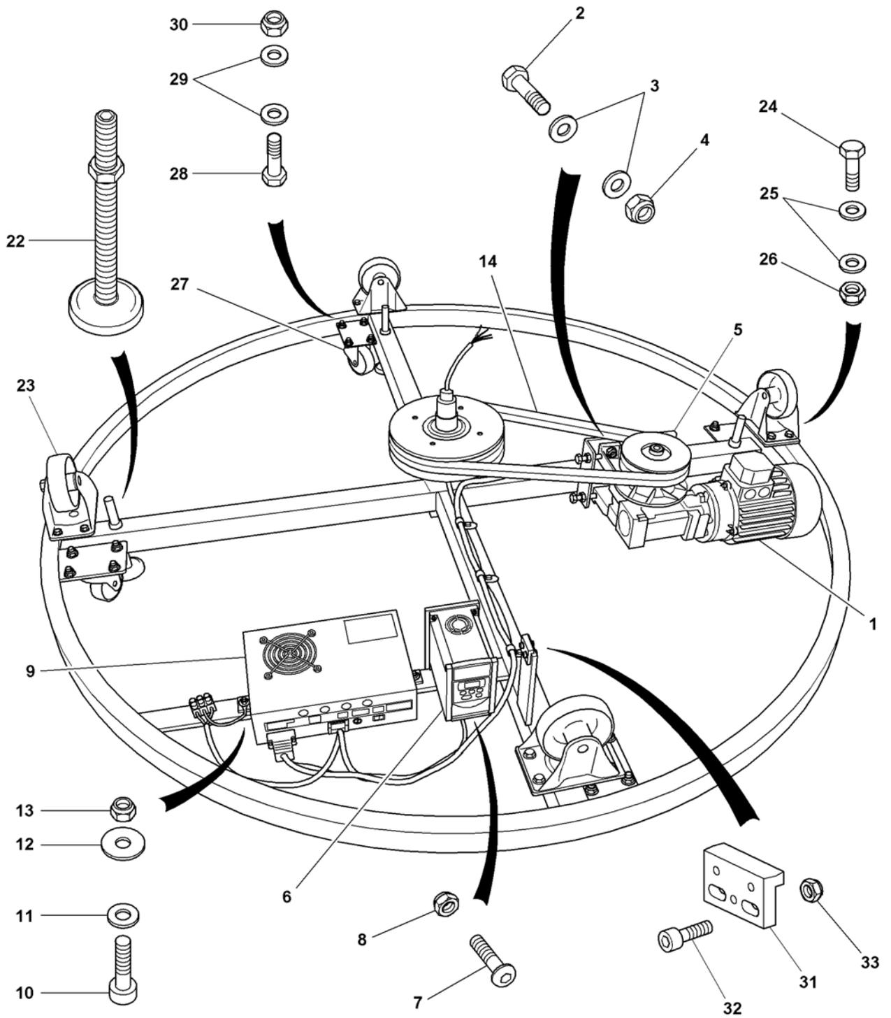
Fig 5 Top and bottom frame assembly
